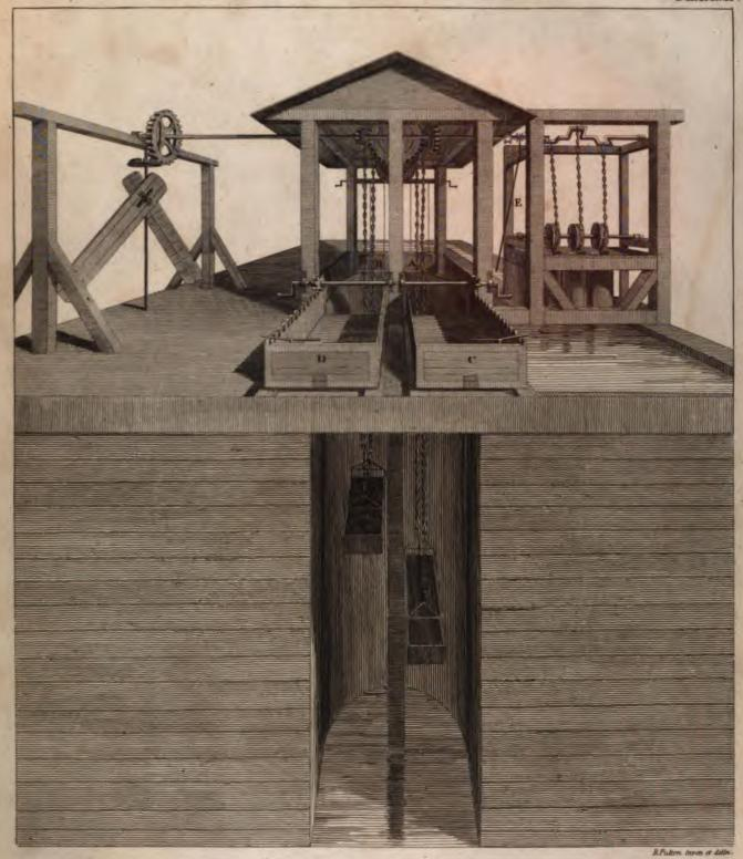
The mode of passing a descending trade and saving the Whole of the Py means of the pumps.
